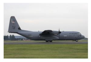
The C-130J is the newest generation of the C-130 Hercules which primarily performs the tactical portion of the airlift mission. The aircraft is capable of operating from rough, dirt strips and is the prime transport for air dropping troops and equipment into hostile areas. The C-130 operates throughout the U.S. Air Force, serving with Air Mobility Command (stateside based), Air Force Special Operations Command, theater commands, Air National Guard and the Air Force Reserve
